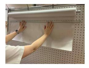
iv. Use two wing nuts to attach the metal ruler to the peg board below the metal pipe so that the newsprint paper rolls underneath it.
